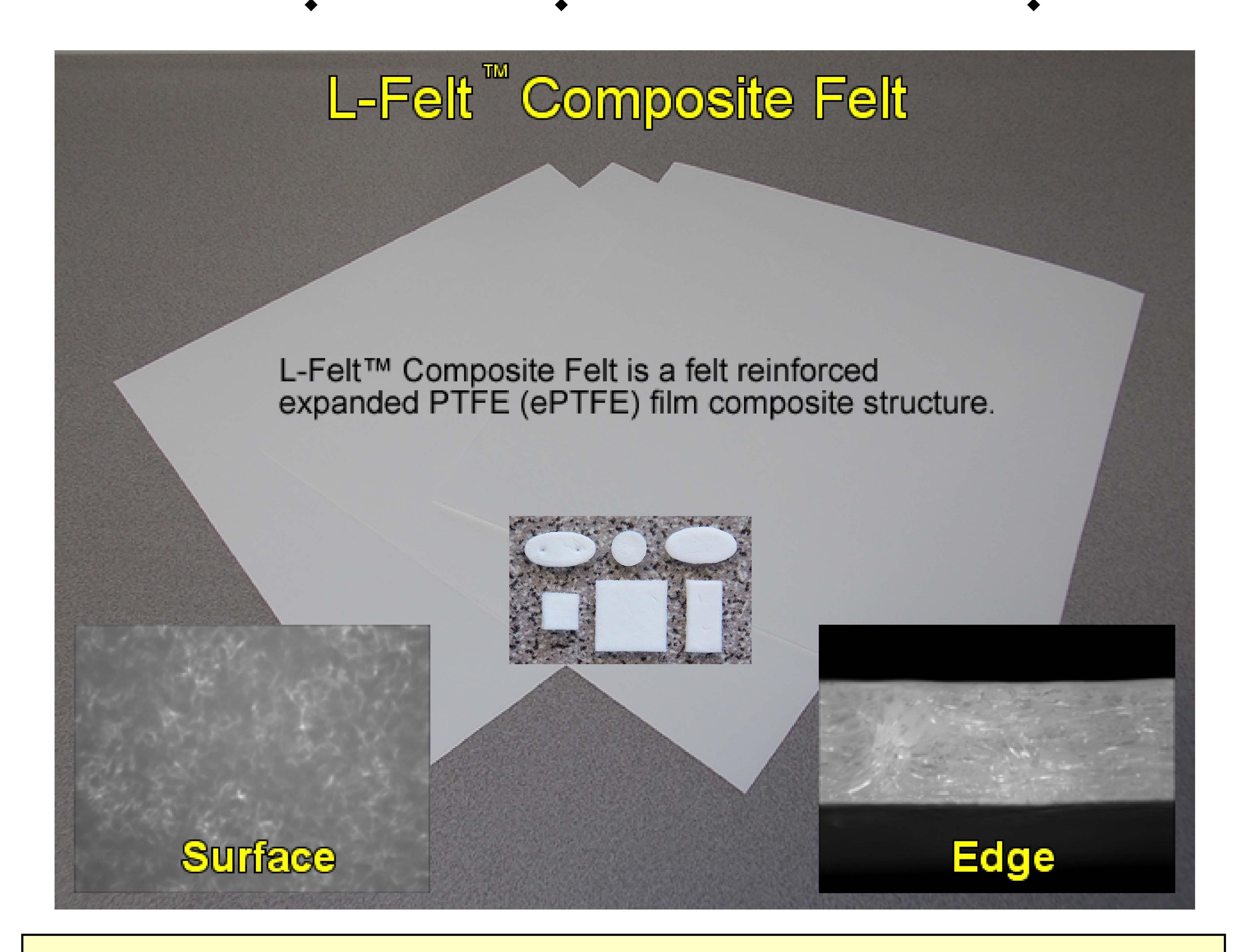
Microporous ePTFE film provides very smooth bonded surfaces, while the felt core provides toughness and strength. The composite felt is ideally suited for the manufacture of suture pledgets due to its low particle shedding propensity, firm hand, toughness, pliability, resiliency and ease of cutting,
