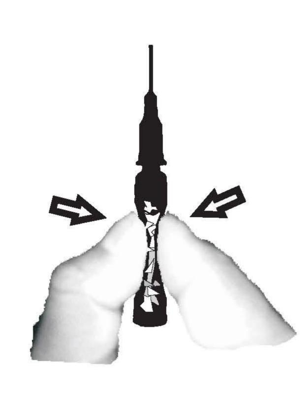
Firmly press in the middle to crush the glass ampule inside
